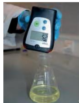
Vapour measurement with an explosimeter
